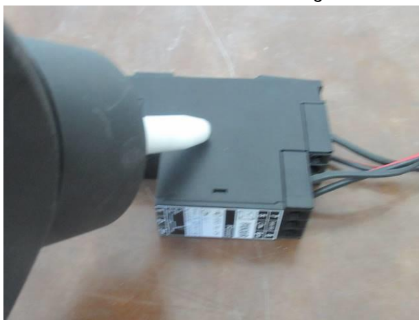
Picture 3.1. A – Air discharge
